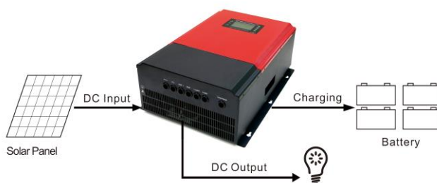
PV Power System Connection Diagram
