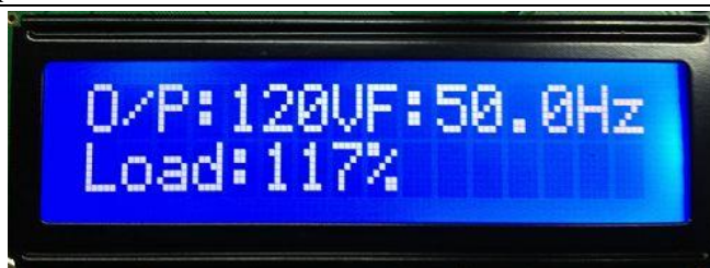
Output Voltage/Frequency and Output Current( in percentage) in Inverter mode
