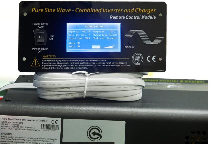
MODE NO; PS W7 3012 DC INPUT : 12VDC AC INPUT: 120VAC 60Hz 30Amax 10
