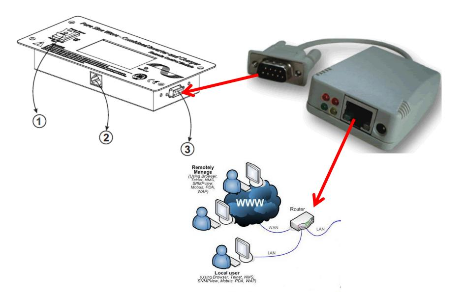
Four: Install the Netility V4.53 software on computer and start remote monitoring. The SNMP card is only capable of monitoring, it can't power on or off the inverter.
